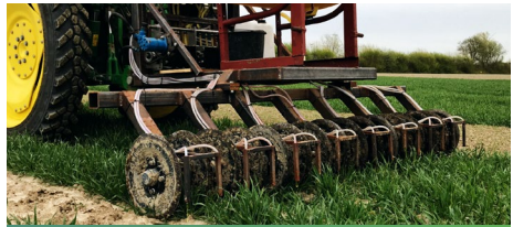
Application of ammonium salts to grass through injection
