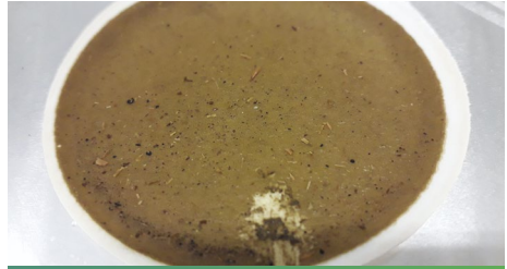
Current stage of struvite refinement, struvite-rich precipitate
